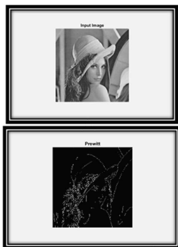
Figure 10. Prewitt edge detection.
